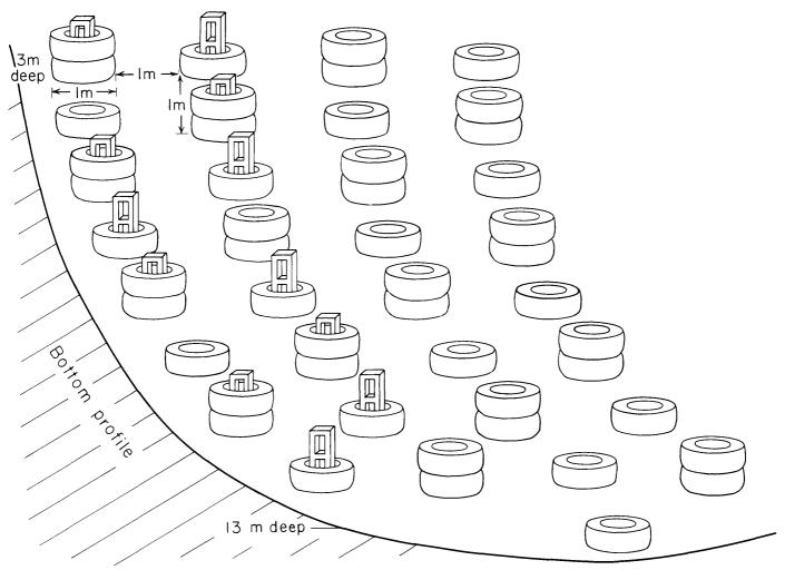
Fig. 1. A schematic view of the artificial habitat showing the matrix of tires, some containing concrete blocks.
