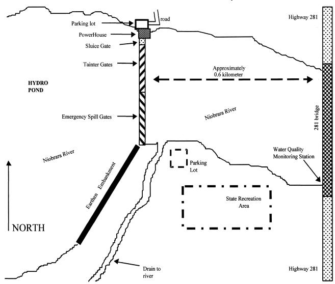
Figure 2. Map of Spencer Hydro structures and dam on the Niobrara River.
