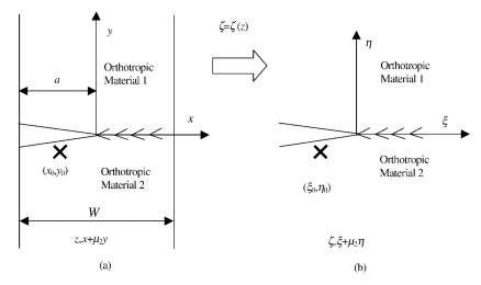
**Figure 1.** A cracked bimaterial under antiplane singularity: (**a**) an edge-cracked bimaterial strip (*z*-plane); (**b**) a semi-infinite interfacial crack between two bonded dissimilar orthotropic half-planes (ζ-plane).
