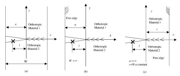
**Figure 2.** A cracked bimaterial with an antiplane point loading applied on the lower crack surface: (a) an edge-cracked bimaterial strip; (b) an interfacial crack between two bonded dissimilar anisotropic quarter-planes; (c) a semi-infinite interfacial crack heading towards a free surface.
