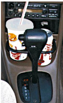
This is the center console in a rental car showing how the cup holder is blocking access to the radio and cassette player. Its nice to have a cup holder, but this isn't a very good spot for it. Not only is it hard to use the radio, but if your drink spills, its going into the cassette player!
