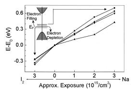
FIG. 3. Binding energy shifts for the occupied and unoccupied molecular orbital features of doped polyaniline, relative to undoped polyaniline, for each experimental deposition step. The symbols  $\blacksquare$ ,  $\nabla$ ,  $\bullet$ , and  $\triangle$  correspond to features A, B, C, and D, respectively in Fig. 2. The approximate exposure is indicated for Na and I2. A schematic of electron filling and depletion is shown in the inset.
