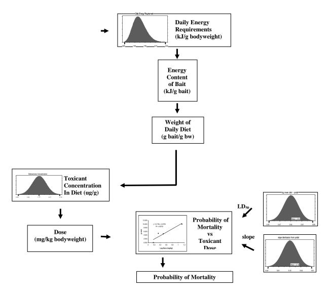
Figure 4. Computer model flow chart.
