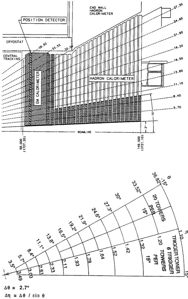
FIG. 2. Cross section of upper part of plug calorimeter (top), and transverse segmentation, showing physical and trigger towers in a  $30^\circ \phi$  section (bottom). The logical segmentation for clustering purposes is the same except in the outer two rings ( $\theta > 30^\circ$ ), where two neighboring (in azimuth)  $7.5^\circ$  towers are merged to match the 15 segmentation of the central and wall calorimeters behind them.
