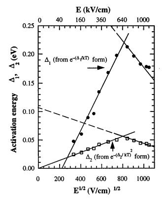
FIG. 3. The activation energy vs  $E^{1/2}$ . The activation energy  $\Delta_1$  is derived assuming the conventional from  $\exp(-\Delta_1/kT)$  form and activation energy  $\Delta_2$  is derived from assuming the  $\exp[-(\Delta_2/kT)^2]$  form appropriate to the Gaussian disorder model.
