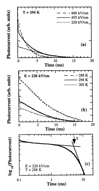
FIG. 1. The time-of-flight photocurrent transients (a) at different fields and at temperature 294 K and, (b) at different temperatures and at field 220 kV/cm. The log-log plot (c) for field 220 kV/cm and temperature 288 K allows determination of the transit time in the presence of strong dispersion.
