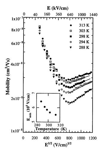
FIG. 2. The logarithm of mobility showing a minimum in the mobility  $E_{\min}$  and the Poole–Frenkel dependence at high fields. The solid lines are fits to Eq. (1). The inset shows the variation of the  $E_{\min}$  with temperature.
