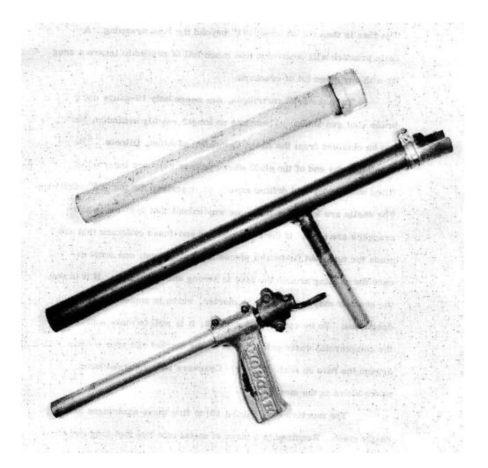
Figure 15 - Three Shell Firing Mortars. The Upper Is Fitzwater's Simple Pipe and Cap. A Hole Drilled in the Cap Permits the Fuse to Stick Out at the Lower End. The Other Two Mortars Are the Same as Shown in Another Illustration Except that a Sheet Metal Shield Has Been Added to Permit Easier Lighting of the Fuse. The Shields Are Sandpaper Lined for Convenience in Striking Matches.
