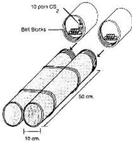
Fig. 1. Diagram of a bait station. ICI Americas Indicator Bait Blocks were wired into the caps on each PVC pipe. CS<sub>2</sub> was associated with the Bait Blocks in one tube.
