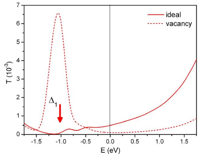
FIG. 3. (Color online) Majority-spin transmission probability vs energy per cell in Fe/MgO/Fe(001) with 5 ML of MgO for ideal MgO and MgO with O vacancies ( $\frac{1}{8}$  cell). The arrow indicates the bottom of the majority  $\Delta_1$  band.
