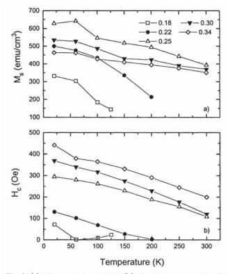
Fig. 2. (a)  $M_s$  versus temperature, (b)  $H_c$  versus temperature for  $Mn_x Pt_{1-x}$  (x = 0.18, 0.22, 0.25, 0.30, 0.34).
