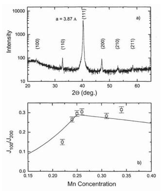
Fig. 1. (a) X-ray diffraction of  $Mn_{0.25}Pt_{0.75}$  thin film; (b) XRD intensity ratio of the (100) to (200) diffraction peaks as a function of Mn concentration.  $\square$  experimental data; solid curve, calculated ratio as discussed in text.
