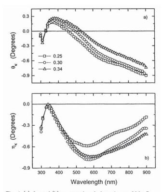
Fig. 4. (a)  $\theta_K$  and (b)  $\eta_K$  wavelength dependence of  $\operatorname{Mn}_x \operatorname{Pt}_{1-x}$  (x = 0.25, 0.30, 0.34).
