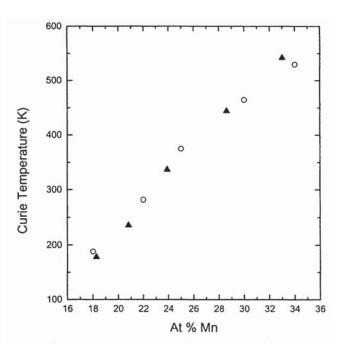
Fig. 3. Curie temperature versus Mn concentration for bulk and thin-film specimens;  $\bigcirc$  thin film,  $\blacktriangle$  bulk [9].
