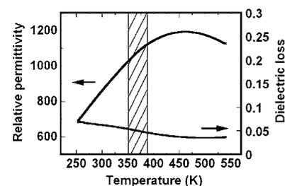
FIG. 4. Temperature dependence of dielectric properties for PLZT (10/65/35) thin films on copper foil. The shadow area shows the  $T_C$  regions for bulk PLZT (Ref. 5) and films on Pt/SiO<sub>2</sub>/Si (Ref. 17).
