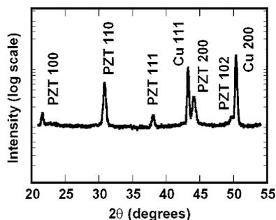
FIG. 2. X-ray diffraction pattern for PLZT (10/65/35) thin film on copper foil.
