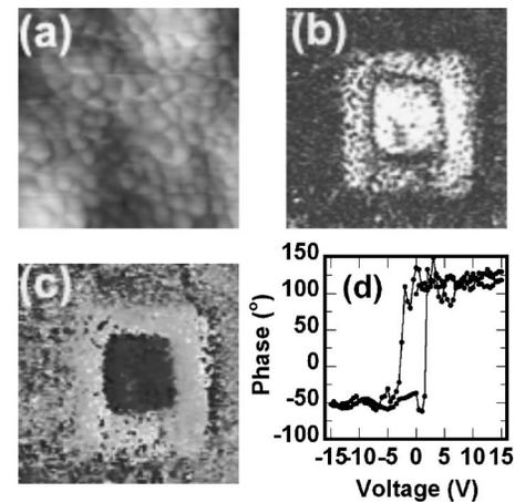
FIG. 3. (a) Topographic ( $2 \times 2 \mu\text{m}^2$ ), (b) amplitude ( $4 \times 4 \mu\text{m}^2$ ), (c) phase ( $4 \times 4 \mu\text{m}^2$ ) images, and (d) piezoelectric phase loop of PLZT (10/65/35) thin films on copper foil.
