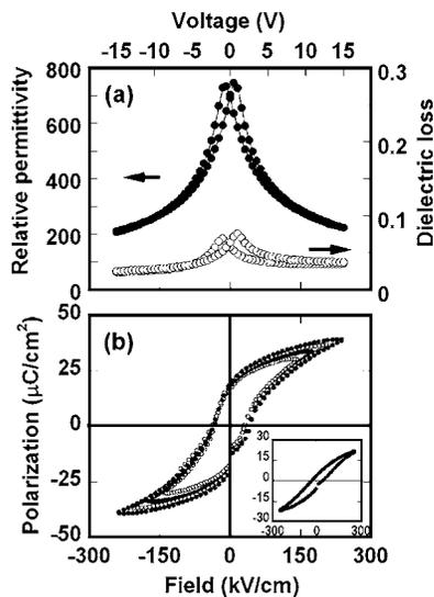
FIG. 1. Field dependent (a) permittivity and dielectric loss and (b) polarization for PLZT (10/65/35) thin films on copper foil. The inset in Fig. 1(b) is for PLZT (10/65/35) thin films on Pt/SiO<sub>2</sub>/Si, processed in parallel with PLZT (10/65/35) thin films on copper.
