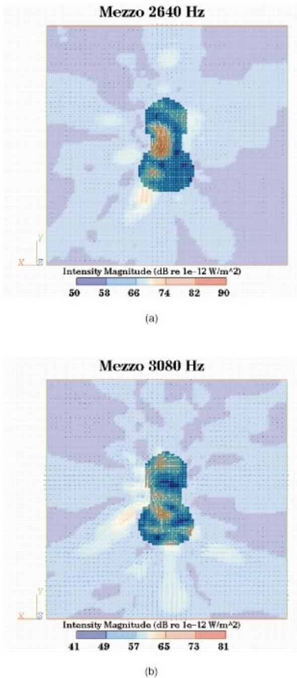
FIG. 14. NAH reconstructed intensity field for the mezzo violin SUS100 facing the back plate at (a) 2640 Hz and (b) 3080 Hz. The plotted data are from the closest local  $z$  plane that does not intersect the violin surface. The three-dimensional intensity vectors are shown, while the intensity vector magnitudes are denoted by color.
