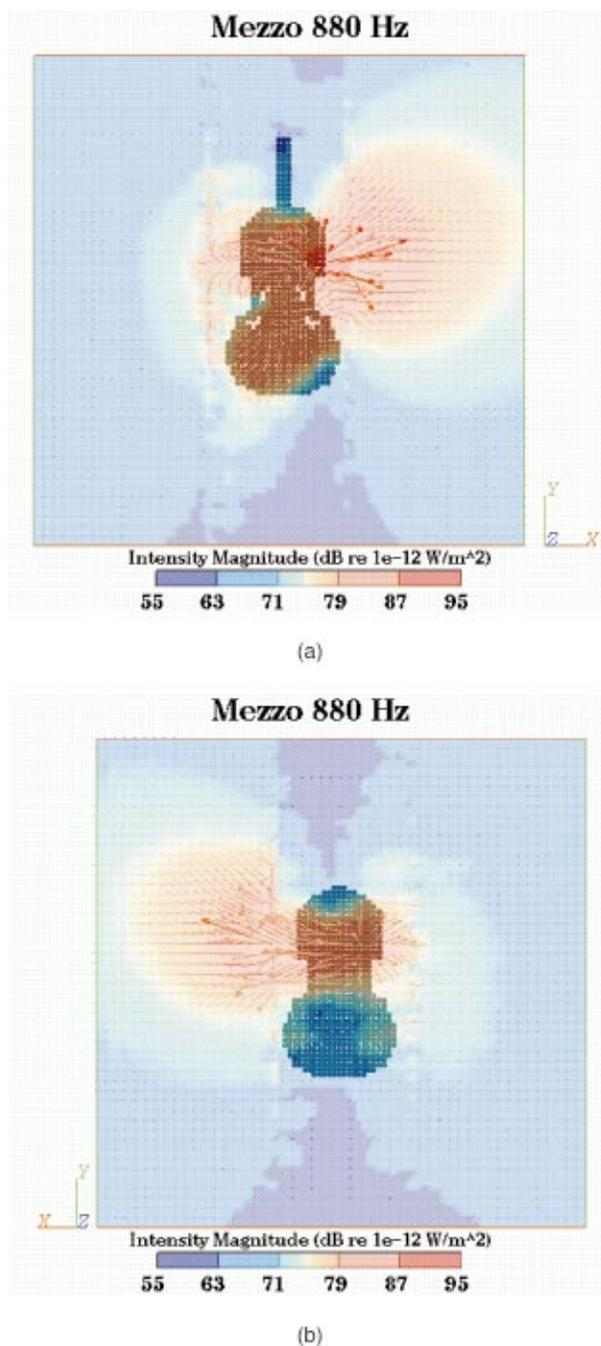
FIG. 11. NAH reconstructed intensity field for the mezzo violin SUS100 at 880 Hz: (a) facing the top plate and (b) facing the back plate. The plotted data are from the closest local  $z$  plane that does not intersect the violin surface. The three-dimensional intensity vectors are shown, while the intensity vector magnitudes are denoted by color.
