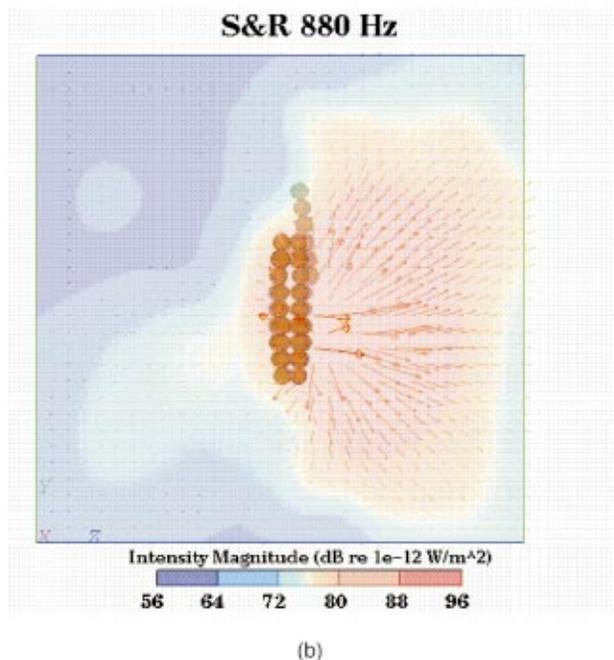
FIG. 6. NAH reconstructed intensity field for the Scherl and Roth violin at 880 Hz: (a) facing the top plate and (b) facing the bass bar side. The plotted data are from the closest local  $z$  plane that does not intersect the violin surface. The three-dimensional intensity vectors are shown, while the intensity vector magnitudes are denoted by color.
