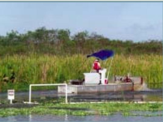
*Entrance fee money collected at A.R.M. Loxahatchee NWR, FL, has helped support a “cookiecutter,” or floating mechanical trail cutter. It maintains 5.5 miles of canoe trail. Its two rotating blades cut the submerged and floating vegetation, clearing the trail for paddlers. (USFWS)*
