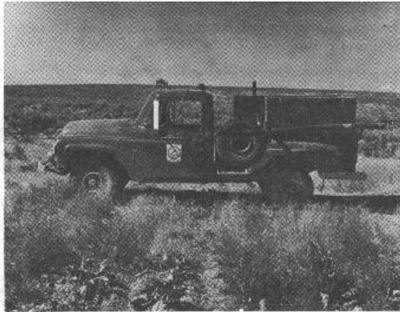
Fig. 2. Bottom end of tube is set in a bracket to permit travel without detaching bait dispenser.
