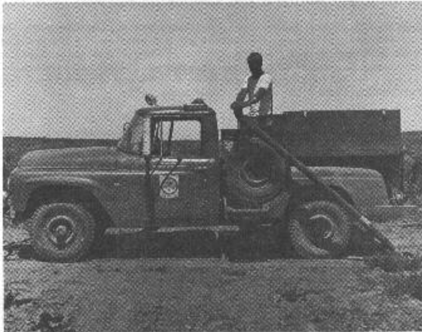
Fig. 3. In baiting operations, carrots are transferred from container to tube by operator. Baiting rate is regulated by speed of the vehicle.
