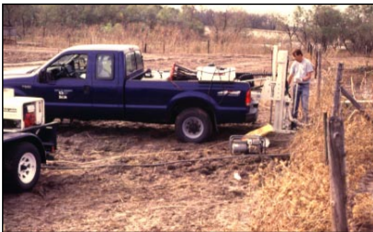
UNL Water Sciences Laboratory Research Technician Jeff Toavs uses a Geoprobe to gather groundwater samples near a confined animal feeding operation (CAFO) waste lagoon as part of a UNL Water Sciences Laboratory study to determine livestock waste lagoon contributions to groundwater pollution. Lagoons and the groundwater near them were sampled for a wide variety of potential pollutants (photo: Mark Burbach).
