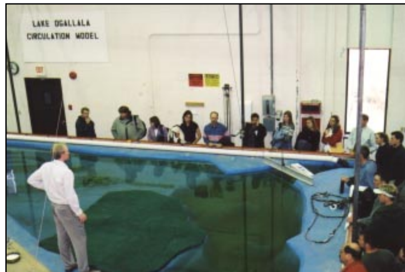
David Admiraal (left), assistant professor in the UNL Department of Civil Engineering, explains the workings of a model of Lake Ogallala that is being used in a multi-disciplinary study aimed at finding solutions to low dissolved oxygen levels in the lake that contribute to fish kills. Admiraal gave the presentation as part of the UNL Water Center's spring semester water and natural resources seminar series (photo: Steve Ress).
