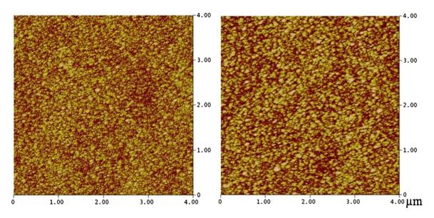
FIG. 1. (Color online) AFM images for BC (left) and Ni(9)-BC (right) on Si substrates, showing no significant change in the surface quality. rms roughness values are 2.1 nm for BC and 2.5 nm for Ni(9)-BC. The z range is 15 nm.
