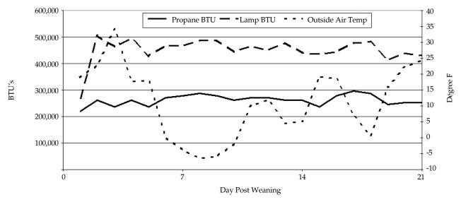
Figure 3. Daily energy usage (Btu's) for each heating system and 24 hour average outside air temperature.
