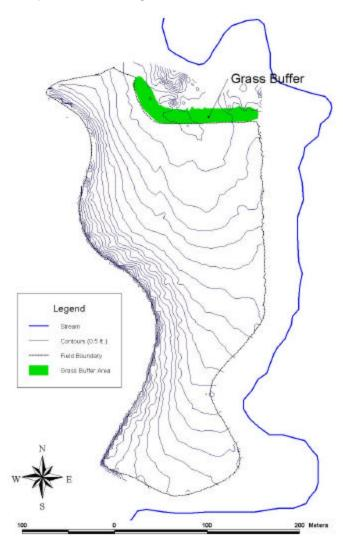
**Figure 1:** Topographic map produced from the laser/GPS survey.
