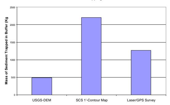
**Figure 5:** Predicted sediment trapping in a buffer using three topographic data sources.
