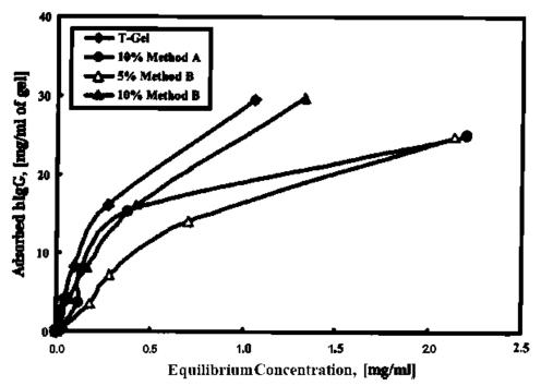
FIGURE 1 Static adsorption isotherms for T-gel and thiophilic cellulose beads. Thiophilic cellulose beads and T-gel beads were contacted with different concentrations for htgG as described in the methods section. The equilibrium concentrations were measured spectrophotometrically at 280 nm. The amount of htgG bound was determined by difference. All experiments were carried out at room temperature. A representative set of isotherms is shown
