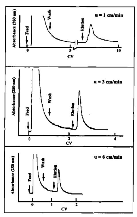
FIGURE 2 Purification of human IgG from a human serum on thiophilic cellulose beads. Beads were packed in 12 cm  $\times$  1 cm i.d columns. The linear velocity is shown on each diagram. Sample loading and column wash buffer was 0.5 M  $\rm K_2SO_4$ , 50 mM  $\rm NaPO_4$  pH = 8.0. Elution of bound IgG was achieved by a step change to 50 mM  $\rm NaPO_4$  pH = 8.0. All columns were operated at temperature 4 °C; detection was performed at 280 nm. Sample feed was 1.5 ml of human serum
