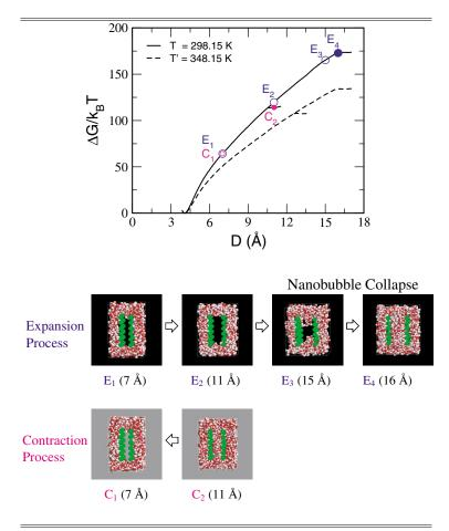
FIG. 2 (color). The calculated PMF curve ( $\Delta G/k_BT$  vs the interhydrophobe distance D) for two  $6\times 6$  hydrophobes in the expansion and the contraction process. The open circles highlight the stable nanobubble state, whereas the solid circles highlight the nanobubble-collapsing state. Snapshots corresponding to these specific states are displayed.
