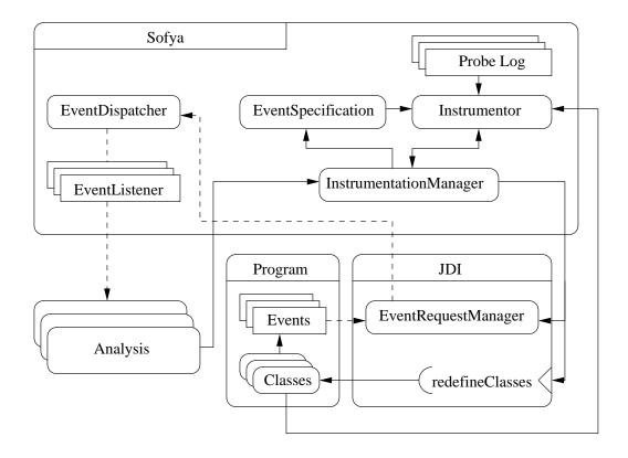
Figure 6: Sofya Adaptive Instrumentation Architecture
