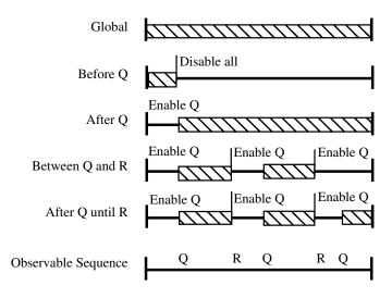
Figure 3: Specification Pattern Scopes
