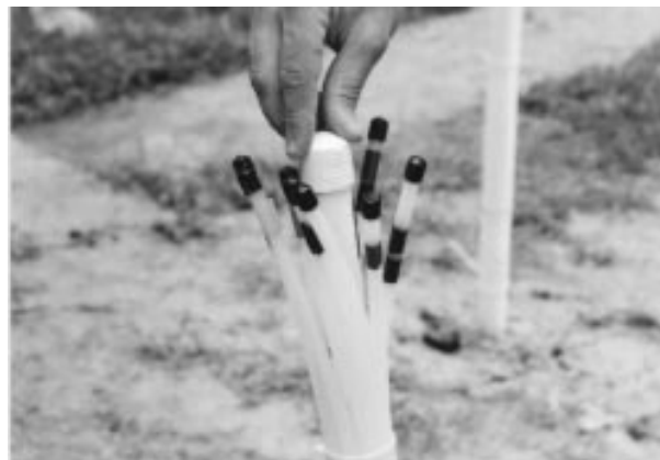
Monitoring wells are included in the daisy well denitrification systems being perfected at the UNL Water Sciences Laboratory (photo: Steve Ress).
