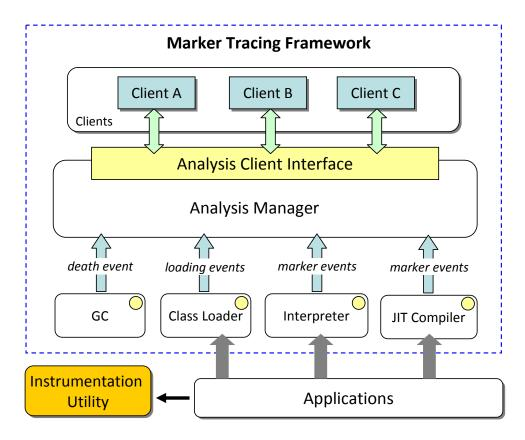
Figure 3.1: Overall architecture of MTF.
