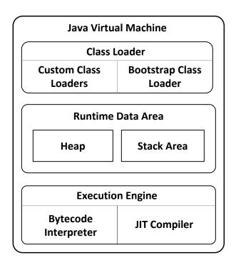
Figure 2.1: Overview of the architecture of a JVM.
