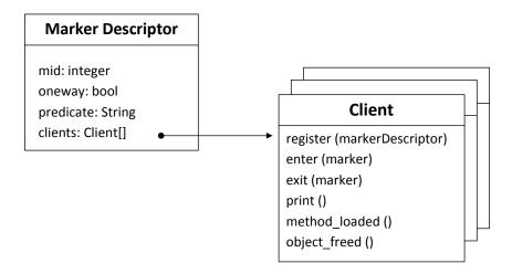
Figure 3.3: The structure of a marker descriptor.
