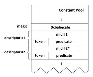
Figure 3.13: Layout of the constant pool after instrumentation.
