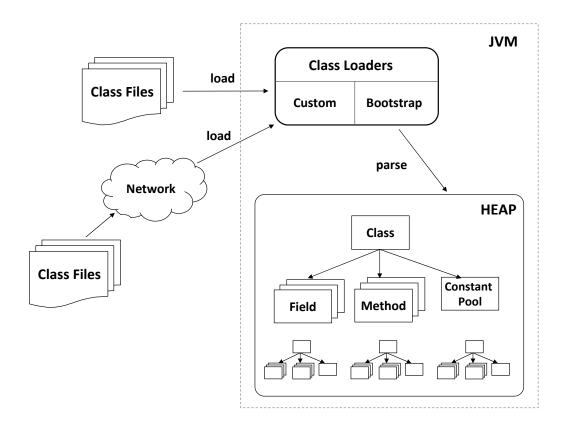
Figure 2.3: Class loaders in a JVM.
