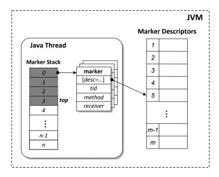
Figure 3.4: Per-thread marker stack
