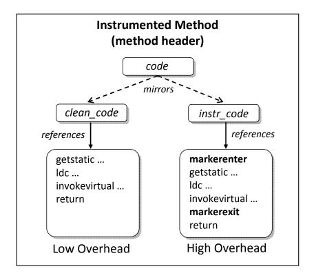
Figure 3.5: Adaptive online program analysis: the MPS approach.
