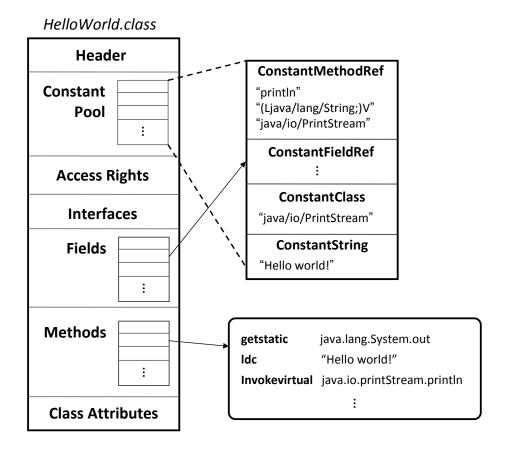
Figure 2.2: The structure of a Java class file.
