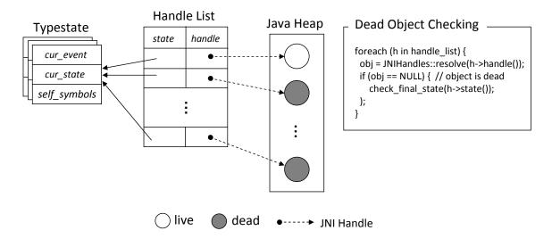
Figure 4.3: Dead object typestate checking.
