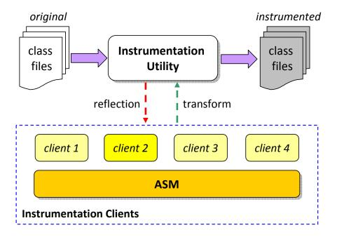
Figure 3.8: Workflow of marker instrumentation.
