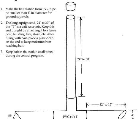
Fig. 5. Commonly used inverted "T" ground squirrel bait station made of 4-inch (10-cm) PVC pipe. Stake secures station in upright position.
