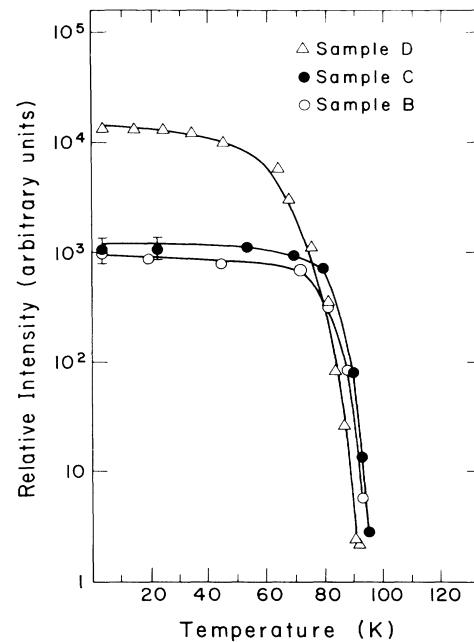
FIG. 3. The temperature dependence of the magnitude of the zero-field absorption. ○: multiphase sample B. ●: multiphase sample C. △: single-phase sample D.
