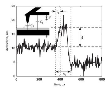
Fig. 2. A representative temporal dependence of the tip deflection from 30 nm thick PS film ( $M_{\rm W}{\sim}110\,{\rm k}$ ). The tip was biased at  $-41\,{\rm V}$  for 280 µs using rectangular pulse shape starting at 360 µs as indicated by the dotted vertical line. The rise time of the voltage source is below 5 µs. Inset: a schematic presentation of the two-capacitor system formed by tip-dielectric-conductor, and lever-dielectric-conductor layers.
