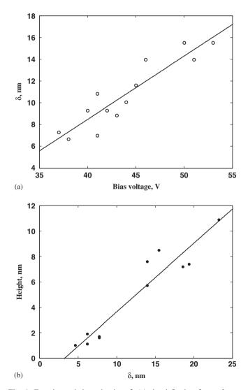
Fig. 4. Experimental dependencies of: (a) the deflection factor  $\delta$  as a function of the bias voltage V; (b) nanostructure height patterned in polymer film versus deflection factor  $\delta$  for PS (30 nm thick film,  $M_{\rm W}{\sim}110\,{\rm k}$ ). The values of  $\delta$  were determined from the deflection signal transients presented in Fig. 2.
