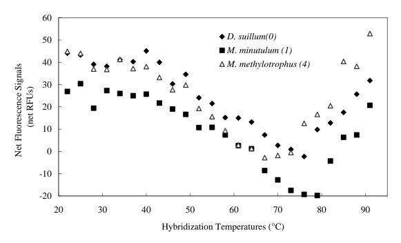
Figure S1. Melting profiles of the hybridization signals of PNA MB Dsoma0848 with its target and non-target 16S rRNAs. The numbers in parentheses indicate the number of mismatches between 16S rRNA and PNA MB.
