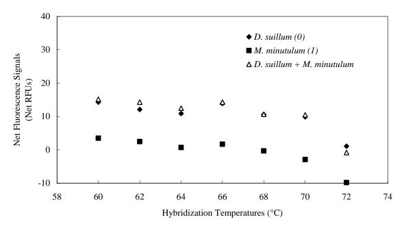
Figure S2. Melting profiles of the hybridization of PNA MB Dsoma0848 with 16S rRNA of its target, non-target, and an artificial mixture of the target and non-target 16S rRNAs. The numbers in parentheses indicate the number of mismatches between 16S rRNA and PNA MB.
