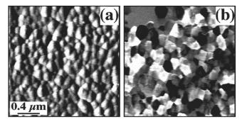
FIG. 1. Topographic (a) and piezoresponse (b) images of the PTO film. White and black regions in the piezoresponse image correspond to positive and negative domains, respectively.
