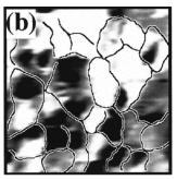
FIG. 6. PFM images of the film subjected to UV/-1 V treatment (a) before, and (b) after poling, illustrating domain pinning at the subgrain level. Black lines correspond to the grain boundaries.
