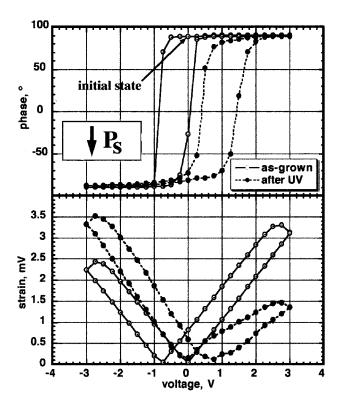
FIG. 3. Phase (a) and amplitude (b) PFM loops of a positively polarized grain before and after UV illumination.
