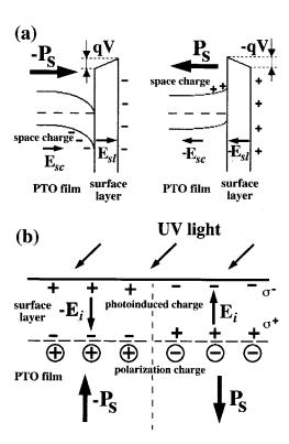
FIG. 4. A band diagram of a ferroelectric with the surface dielectric layer (a) and a schematic diagram (b) illustrating formation of the photogenerated field within the surface dielectric layer under UV illumination.
