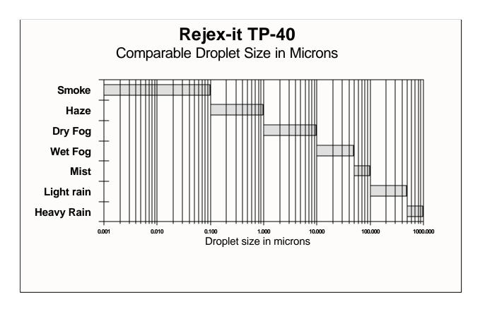
Figure 1. Comparable droplet sizes for Rejex-it® TP-40 versus water.
