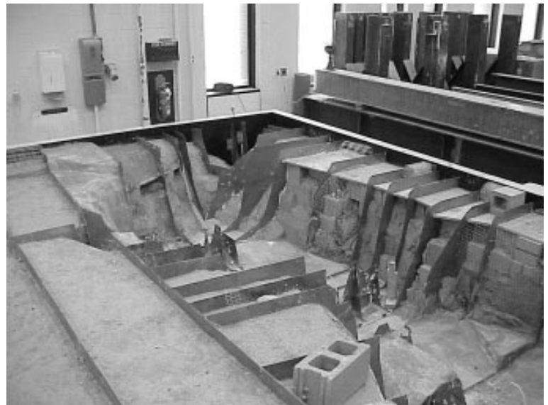
This photograph from the early construction stages of the model of Lake Ogallala clearly shows the hand-cut steel plates, concrete blocks and fill sand used in its construction (photo: Cory Haberman).
