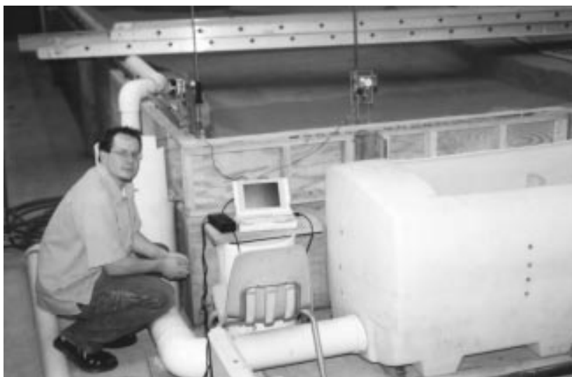
Cory Haberman with the collection tank and computer hardware used in connection with the model of Lake Ogallala to record flow data for researchers (photo: Steve Ress).
