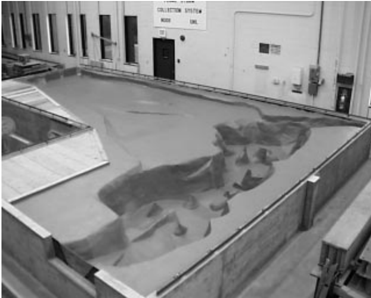
An overhead view of the Lake Ogallala model in the engineering basin of UNL's Walter Scott Engineering building (photo: Cory Haberman)
