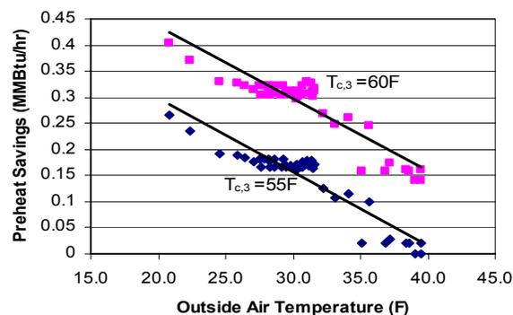
Figure 5: Preheat Energy Savings for LAHU Economizer Operation
