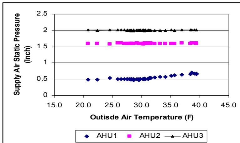
Figure 6: Static Pressure for LAHU Economizer Operation
