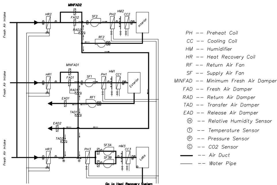
Figure 3. Schematic Diagram of Major HVAC Systems
