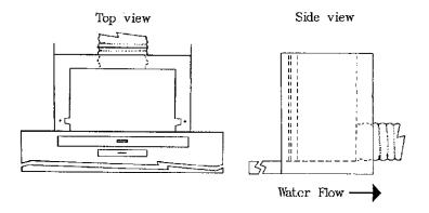
**Fig. 2.** Stoplog (a) and screw gate (b) water-control structures for manipulating water levels.
