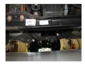
Figure 2.4: SmartWave Receiver/Gateway Mounted on Transmission Lower Crossmember (NHTSA, 2010)
