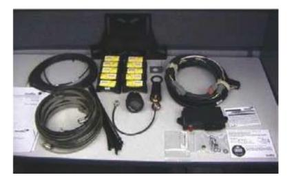
Figure 2.2: Components Kit for SmartWave 10-Tire system (NHTSA, 2010)
