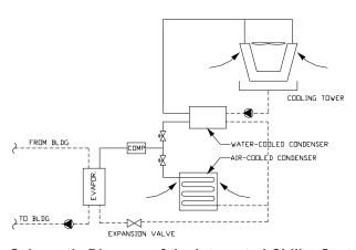
Figure1: Schematic Diagram of the Integrated Chiller System
