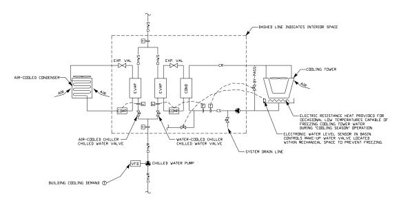
Figure 2: Systematic Diagram of the Integrated Chiller System Implementation in the Case Study
