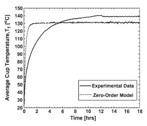
**Figure 8.** A graph presenting the experimental average cup temperature history along with the zero-order model prediction. [Data taken from experiment 13: quiescent air, 133,447 N (30,000 lb) load, steel cages, total heat input of 665.4 W.]
