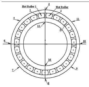
**Figure 4.** A schematic diagram showing the locations of the thermocouples on the bearing assembly. Thermocouples 1, 2, and 3 are attached to rollers, thermocouples 4–11 are fixed to the bearing cup, and thermocouples 12 and 16 are placed at the upper and lower contact areas between the inner cone and the axle, respectively.
