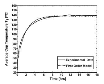
**Figure 10.** A graph presenting the experimental average cup temperature history along with the first-order model prediction. [Data taken from experiment 13: quiescent air, 133,447 N (30,000 lb) load, steel cages, total heat input of 665.4 W.]
