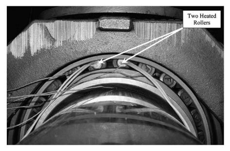
Figure 3. Close-up view of the two heated rollers used to provide known heat inputs to the bearing assembly.
