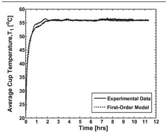
**Figure 9.** A graph presenting the experimental average cup temperature history along with the first-order model prediction. [Data taken from experiment 5: air blowing at 5 m/s (11.2 mph), 133,447 N (30,000 lb) load, steel cages, total heat input of 645 W].
