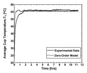
**Figure 7.** A graph presenting the experimental average cup temperature history along with the zero-order model prediction. [Data taken from experiment 5: air blowing at 5 m/s (11.2 mph), 133,447 N (30,000 lb) load, steel cages, total heat input of 645 W.]
