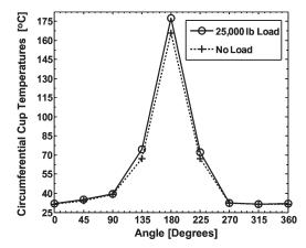
**Figure 11.** A plot of the circumferential cup temperatures comparing the temperature distribution under loading and unloading conditions. [Data taken from experiment 12: air blowing at 5 m/s (11.2 mi/h), 0–111,206 N (0–25,000 lb) varied load, steel cages, total heat input of 653.8 W.]
