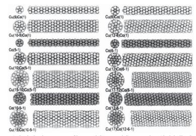
**Figure 1.** Optimized structures of bare and Cu-coated Co nanowires (dark balls: Co atoms; bright balls, Cu atoms). Left part is for the centered hexagonal multishell structural pattern and right one for the centered pentagonal one. The indexes of n-nl-n2-n3 in parenthesis are used to characterize each structure [111].
