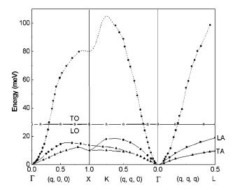
FIG. 3. Dispersion curves for magnons  $(\bullet)$ , longitudinal phonons  $(\blacksquare)$ , and transversal phonons  $(\blacktriangle)$  at 300 K. No magnetic field was applied.
