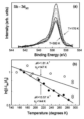
FIG. 2. (a) Normal x-ray photoemission spectra of Sb $-3d_{3/2}$  core level for various temperatures after background subtraction. The light was incident at 60° with a photon energy of 1254 eV. (b) Logarithm of the intensity of the Sb $-3d_{3/2}$  core level vs temperature ( $\bullet$ ) and the intensity of the state at the conduction band edge (just above  $E_F$ ) in inverse photoemission ( $\bigcirc$ ).
