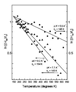
FIG. 1. Logarithm of the intensities of the diffracted electron spots obtained in LEED, after background  $(I_{bk})$  subtraction and normalization to the value  $(I_0)$  at the lowest temperature. The three sets of data were obtained using different incident electron energies: 33 (circles), 58 (up triangle), and 83 eV (diamond).
