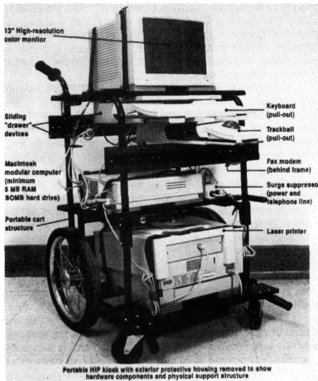
Figure 1. Portable HIP kiosk with exterior protective housing removed to show arrangement of hardware components and the physical support structure.
