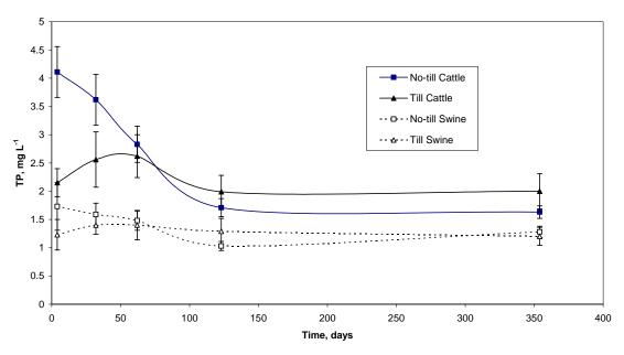
Figure 2c. Total phosphorus (TP) concentrations of runoff versus time since manure application for the experimental treatments. Vertical bars represent one standard deviation of the mean value.
