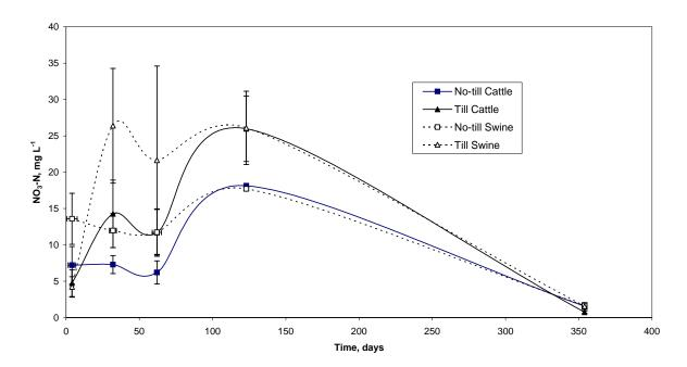
Figure 3a. NO<sub>3</sub>-N concentrations of runoff versus time since manure application for the experimental treatments. Vertical bars represent one standard deviation of the mean value.
