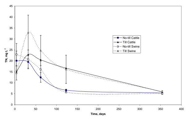
Figure 3c. Total nitrogen (TN) concentrations of runoff versus time since manure application for the experimental treatments. Vertical bars represent one standard deviation of the mean value.
