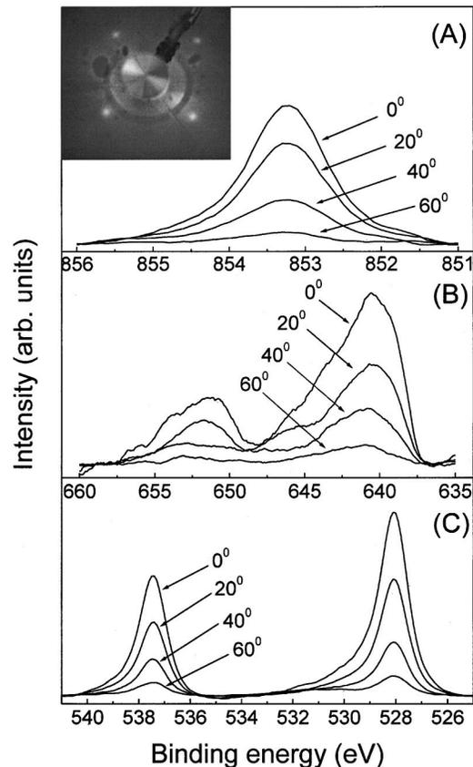
FIG. 1. The emission angle dependence of the x-ray photoemission data. The Ni  $2p_{3/2}$  (A), Mn  $2p_{3/2} + 2p_{1/2}$  (B), and Sb  $3d_{5/2} + 3d_{3/2}$  (C) core levels of NiMnSb are shown as a function of emission angle, as indicated. The LEED pattern of the stoichiometric surface for NiMnSb, obtained at an electron energy of 34 eV is shown in the inset.
