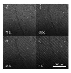
FIG. 8. Magneto-optical images showing the occurrence of a domain state on the micrometer scale which appears as a stripelike variation from bright to dark contrast along the diagonal direction of the sample. This domain state is most pronounced at 5 K and disappears above 65 K.
