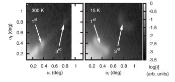
FIG. 7. Off-specular maps at temperature of 300 K (a) and 15 K (b) plotted as a function of the angle of the incident beam,  $\alpha_i$ , versus the one of the reflected beam,  $\alpha_f$ . The significant broadning of the specular signal in (b) arises from the buckling of the sample surface which gives rise to an angular spread of about  $0.3^{\circ}-0.4^{\circ}$ .
