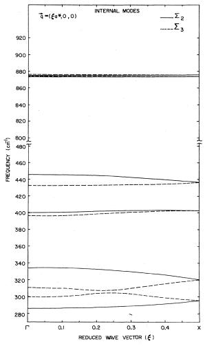
FIG. 6. Phonon dispersion curves for the  $\Sigma_2$  and  $\Sigma_3$  internal vibrations.
