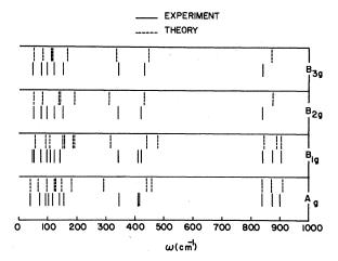
FIG. 2. Observed and calculated Raman frequencies for  $K_2SeO_4$  at 130 K. The observed values are taken from Ref. 18. In every experimental spectrum more lines are seen than are predicted by group theory and we have identified as genuine first-order lines only the most intense lines in any region whose frequencies are those shown in the figure. This criterion reduces the number of lines to the group theoretical value.
