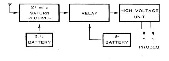
Figure 1. Block diagram of high-voltage collar.
