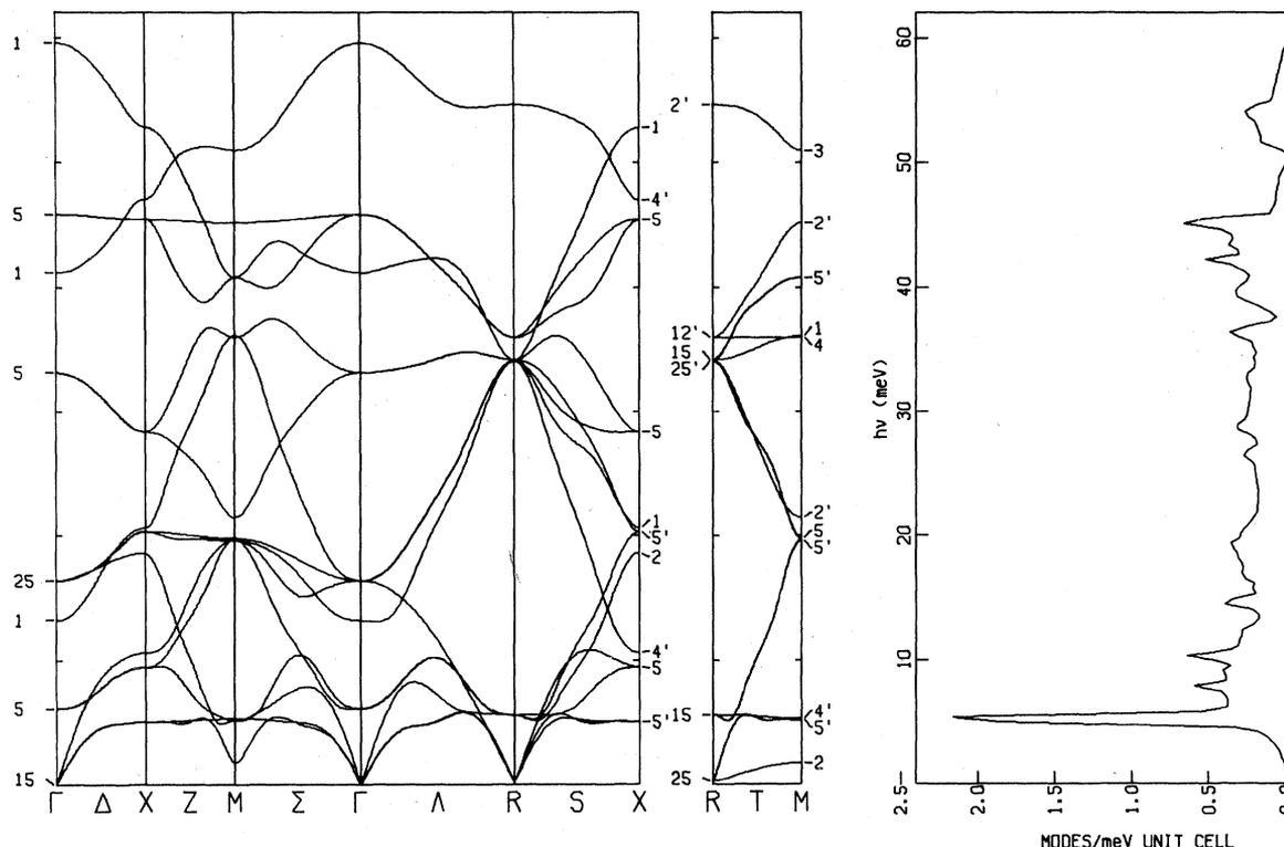
FIG. 8. Quasiharmonic frequency dispersion curves and frequency spectrum for  $\text{RbCaF}_3$  in the perovskite structure at the critical volume ( $b = 8.555$  bohr) below which the  $R_{25}$  frequency is imaginary.
