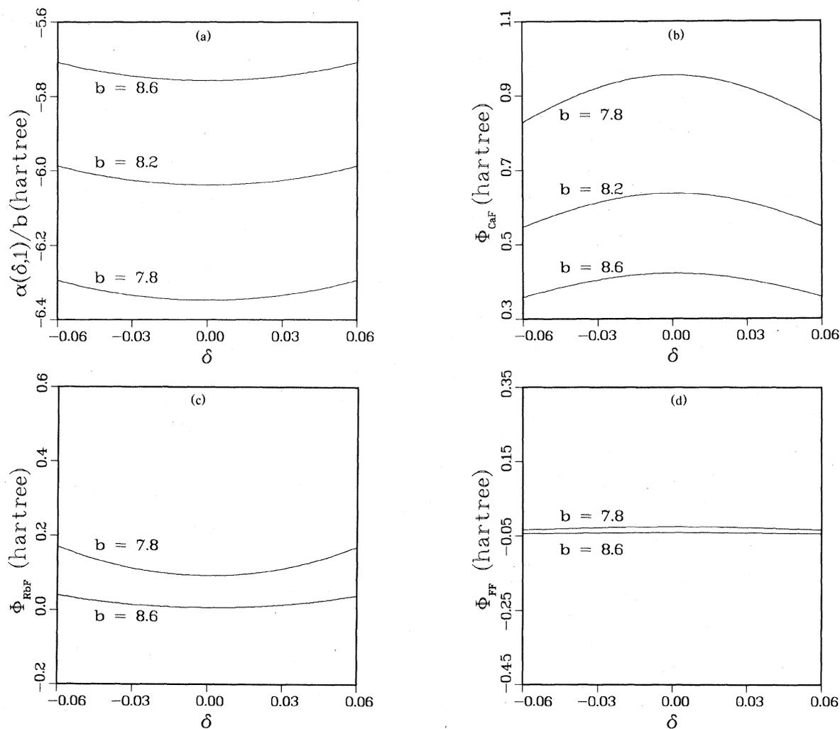
FIG. 6. Separate contributions to the  $\delta$  dependence of the potential energy for selected values of  $b$ , from (a) the long-range Coulomb interaction, (b) the short-range Ca-F interaction, (c) the short-range Rb-F interaction, and (d) the short-range F-F interaction, plotted on a single-energy scale to facilitate comparison of their relative strengths.
