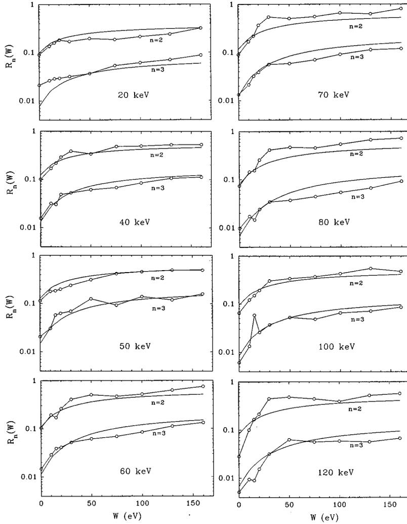
FIG. 5. Charge-state ratios as functions of  $W$ , the ejected electron energy. Points connected by lines, present data ( $W=0$  values are extrapolated; see text); smooth curves, values calculated from Eq. (6).
