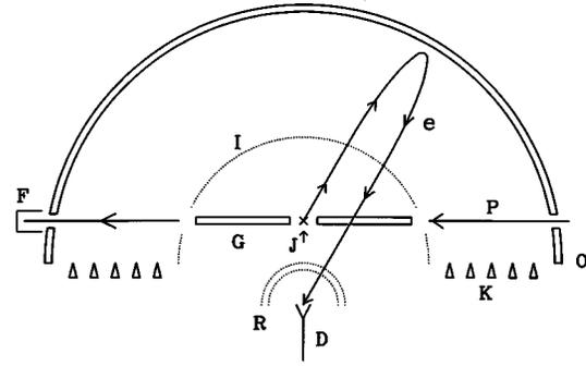
FIG. 2. Schematic diagram of the low-pass high-pass electron energy analyzer.  $P$ , projectile beam;  $G$ , beam guide;  $F$ , Faraday cup;  $J$ , Gas jet;  $e$ , typical electron trajectory;  $I$ , hemispherical grid;  $O$ , outer hemispherical electrode;  $K$ , guard rings;  $R$ , high-pass filter;  $D$ , electron detector.
