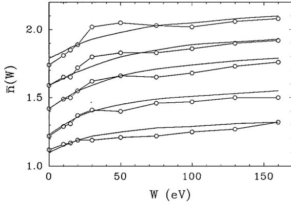
FIG. 6. Comparison of experimental and calculated values of  $\bar{n}(W)$  vs  $W$ . From bottom to top, proton energies are 20, 40, 60, 80, and 120 keV. Values at energies above 20 keV have been shifted upwards by successive amounts of 0.1 to avoid overlap.
