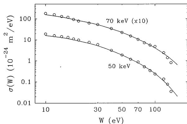
FIG. 3. Noncoincidence electron spectra from 50- and 70-keV  $H^- + Ar$  collisions. Solid lines, SDCS data from Rudd, Toburen, and Stolterfoht [14]; circles, relative SDCS data from this measurement normalized at 50 eV.
