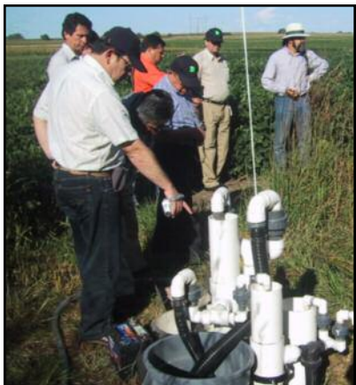
Dr. Dean Eisenhauer shows a runoff sampling station located on field edge and riparian buffer strip to group from Argentina.
