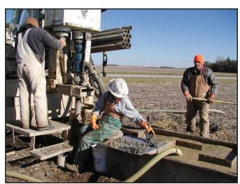
UNL Conservation and Survey Division drilling manager Matt Marxsen, hydrogeologist Sue Lackey and research technician Waylon Hullinger retrieve geologic samples near Oakland. Test holes are typically drilled into the top of bedrock, which in the Oakland area generally occurs between 60 and 260 feet below ground surface (LENRD photo).
