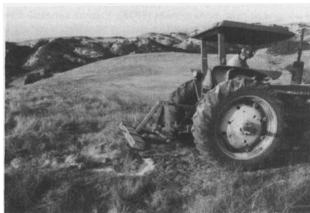
Figure 1. Ripping of squirrel burrows near Livermore, CA. This ripper consists of three 18-in blades. (Note powdered chalk used to delineate the burrow system.)
